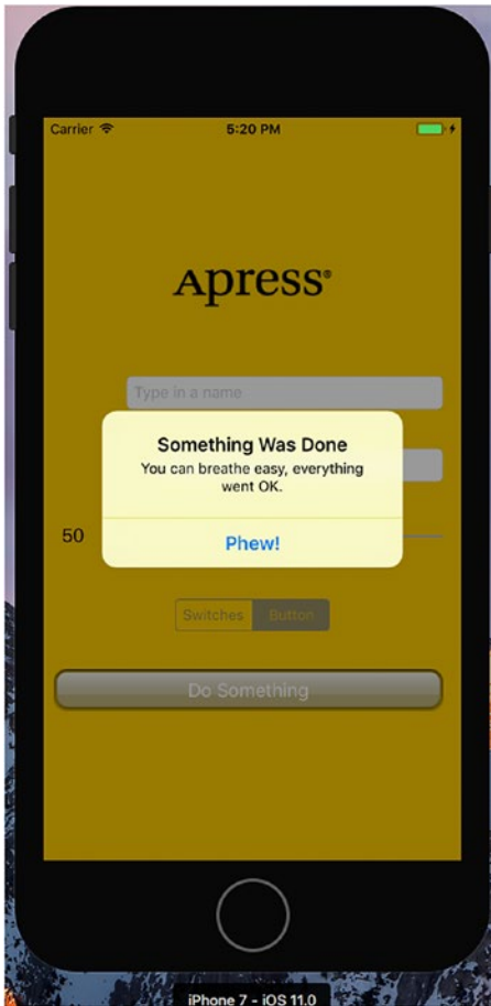
Figure 4-4. Alerts notify the user when important things happen. This app uses one to confirm that everything went OK.
