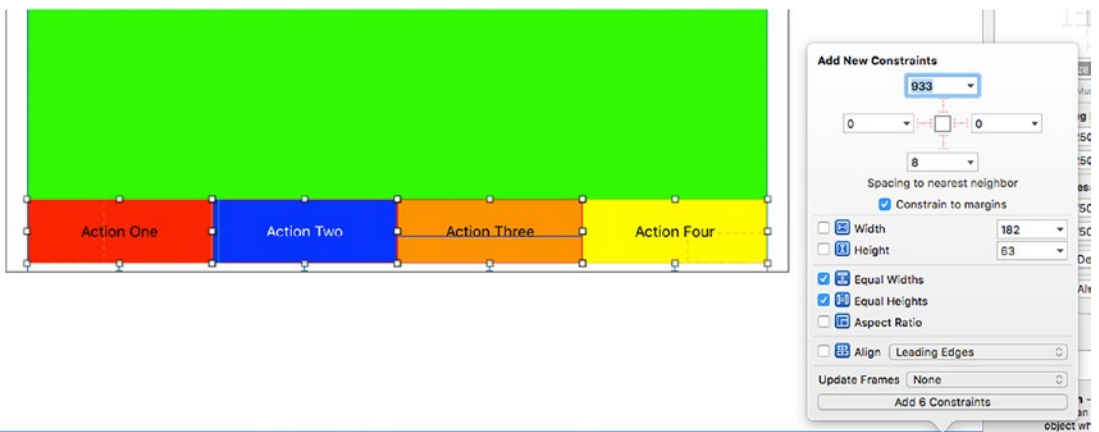
Figure 5-59. Shift-select all four action buttons along the bottom row and set them to equal height and width
