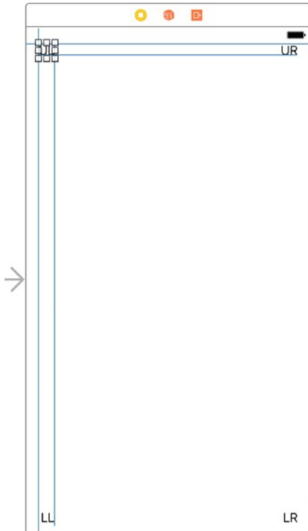
Figure 5-8. The solid blue lines show constraints that are configured for the chosen object
