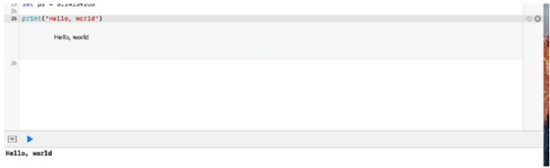
Figure A-5. Viewing output inline with the code and in the debug area
