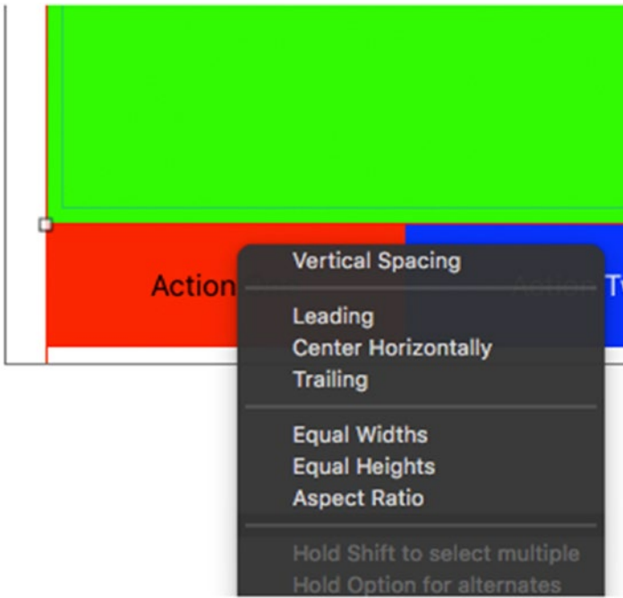
Figure 5-60. Click-drag from the green view to the Action One button and set the vertical spacing. This forces the green view to sit against the row of buttons.
