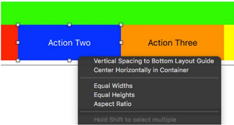
Figure 5-56. Pin the Action Two button to the bottom edge of the containing view
