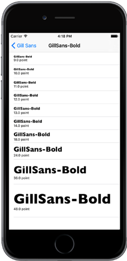
Figure 9-5. Located one layer deeper than the font list view controller, the font sizes view controller shows multiple sizes of the chosen font, one per row
