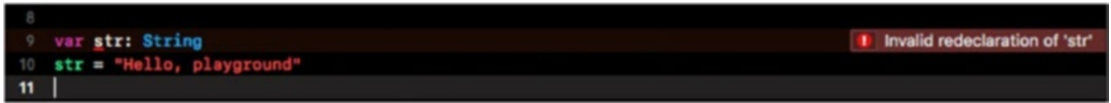
Figure A-4. Swift is not a dynamic language. You can't change the type of a variable.
