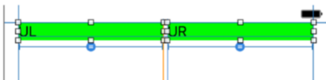
Figure 5-14. The top labels are now made equal in width by a constraint
